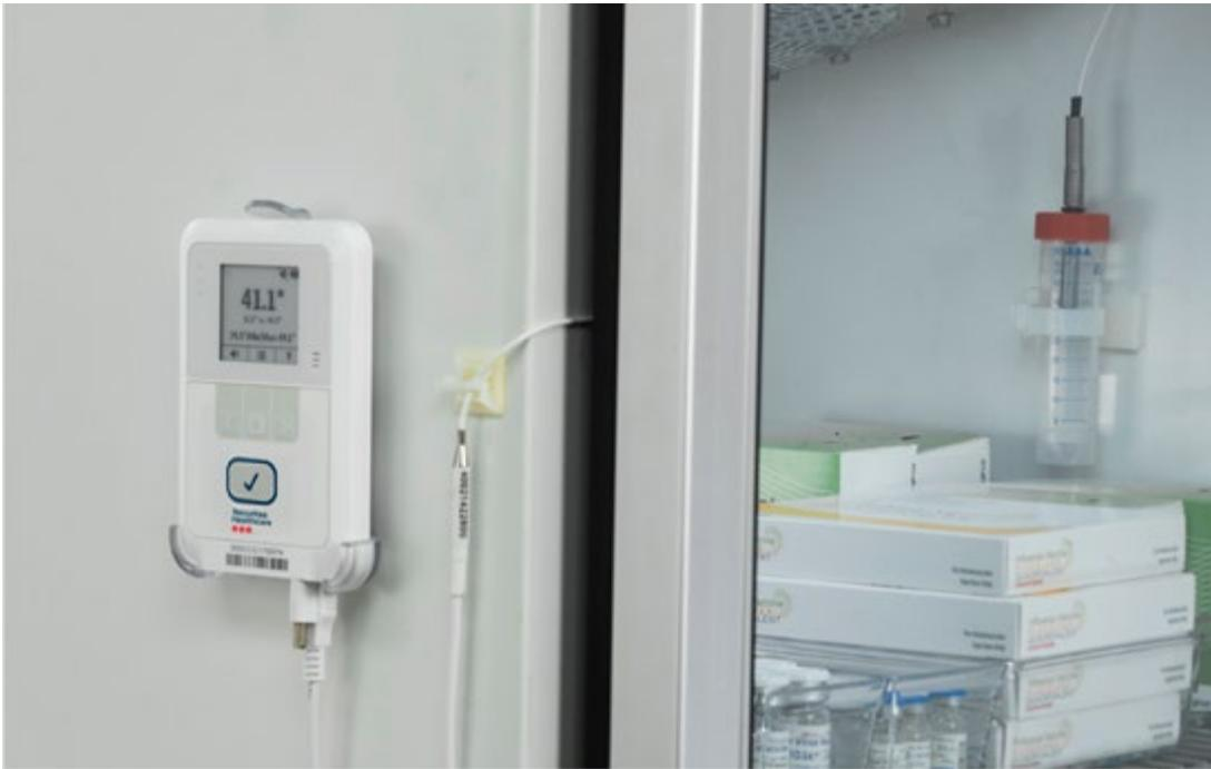
2. Feed the Probe part of the cable (flat section) through the fridge or freezer door seal.
